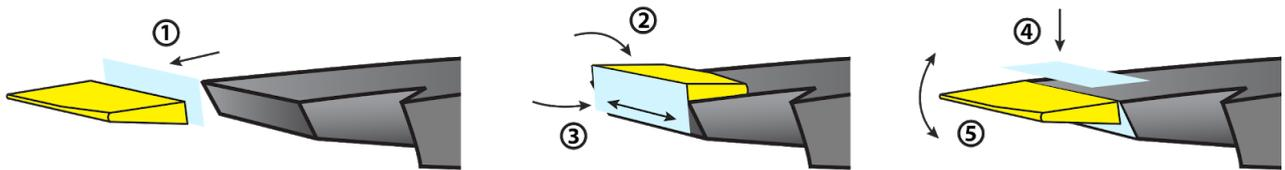
The inner end of the hinges should follow the arc from the frame, in-line with the frame. Leaving a small gap between the winglet and elevon.
