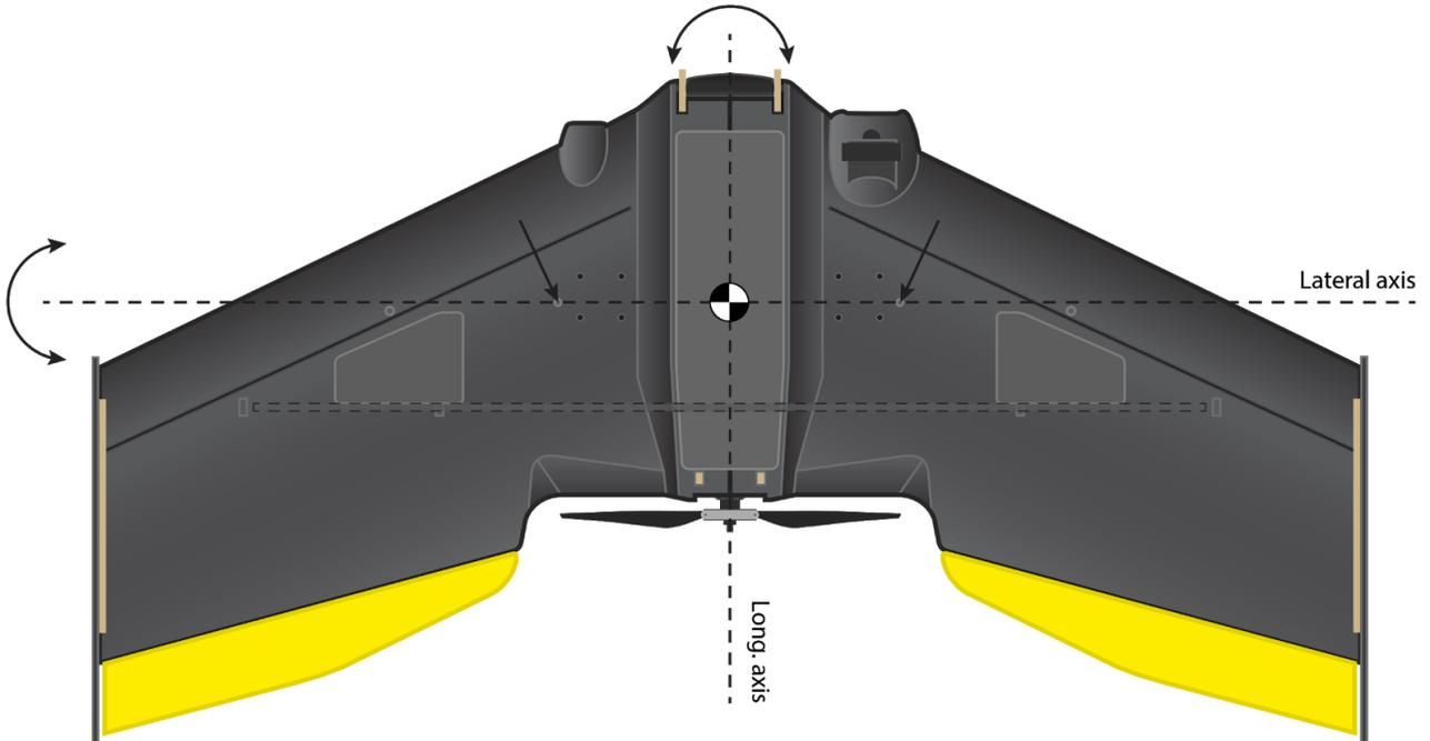
Balance the lateral (pitch) axis within the recommended CG spot. The longitudinal (roll) axis should be balanced straight along the middle of the wing.
